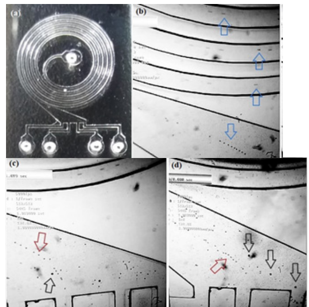
Fig 2. Experimental results: (a) PDMS spiral with four outlets; (b) Microparticles (blue arrows) being transported and focused at the microchannels for a flow rate of 1000 \mu\text{l}/\text{min} ; (c) 20 \mu\text{m} (red arrow) and 40 \mu\text{m} particles (black arrow) both exiting through the same outlet for a flow rate of 1000 \mu\text{l}/\text{min} ; (d) 20 \mu\text{m} (red arrow) and 40 \mu\text{m} particles (black arrow) with separated trajectories exiting through different outlet for a flow rate of 2000 \mu\text{l}/\text{min} .
